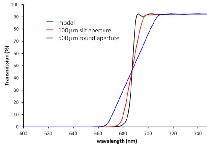
**Figure 5-** Modeled spectra using different aperture sizes and shapes in an  $f/8$  beam. The slit aperture is aligned perpendicular to the spectral- spatial gradient. The gradient in this sample was  $\sim 75$  nm/mm.
