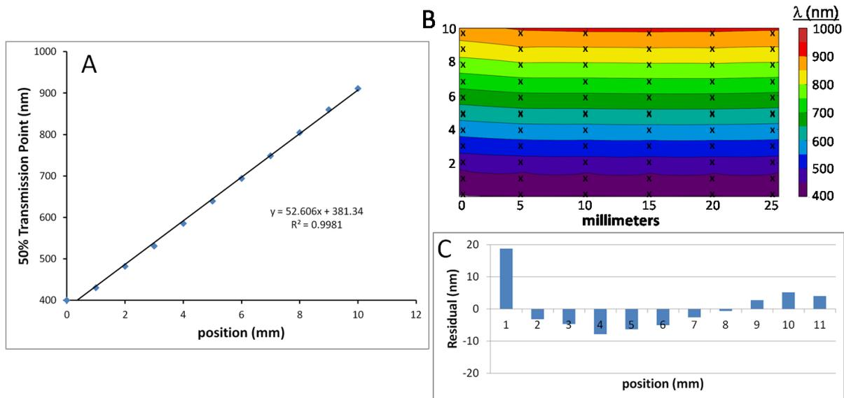
**Figure 3.** High spectral-spatial slope, high-pass LVF under development by Omega Optical. A. Spectral-spatial curve from the 15 mm position, B. Color-coded map of 50% T versus position with measurement positions marked with x, C. Residuals of the line fit from panel A.
