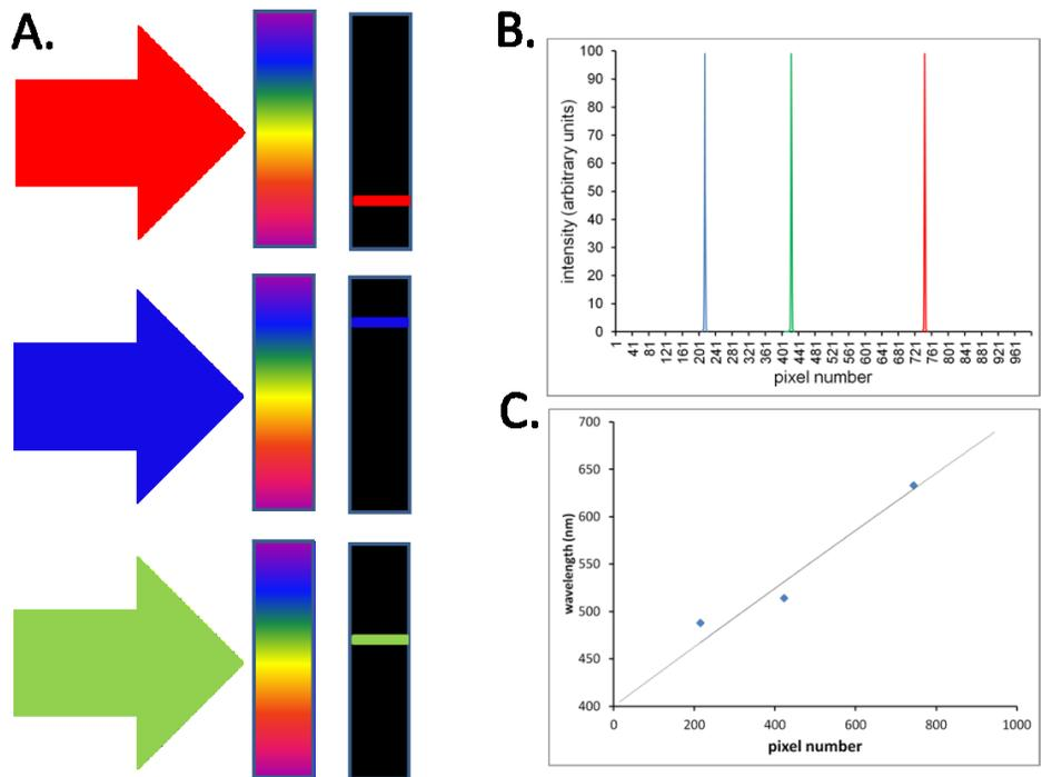
**Figure 6.** A. In the case of a BP LVF, expanded laser lines can be used to align the filter (multicolored rectangle) to the detector (black rectangle), shown graphically in B. C. A plot of pixel number versus laser wavelength is used to generate a calibration curve for the filter/ detector assembly. If the filter exhibits significant smile, a similar curve can be generated for each row of pixels in a 2-D detector and the signals can be combined in software.
