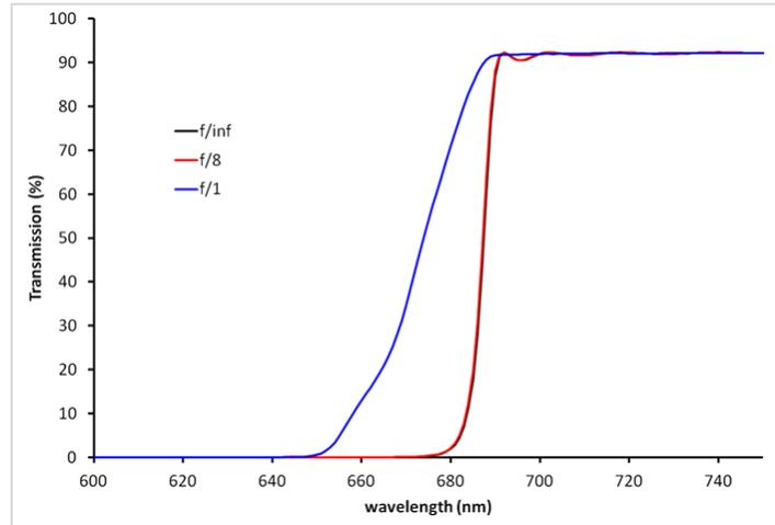
**Figure 4.** Model curves of %T versus wavelength for a single LP filter with AOI=0 and different cone angles ( $f/\#$ ). The increase in cone angle causes a decrease in the slope of the cuton wavelength.
