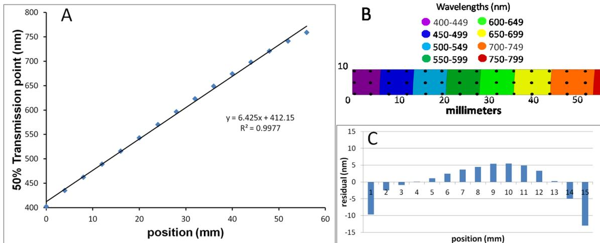
**Figure 2.** Measurements and map from a LP-LVF produced using a mask and rotating platen. A. Spectral-spatial gradient curve from the 5 mm position, B. Color-coded map of the wavelength at 50% T of the LP with measurement positions marked with dots, C. Residuals from the line fit in panel A.
