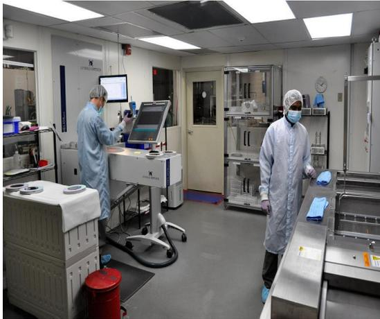
**Figure 18: Parts and product are cleaned and handled in a clean room environment to ensure high yield and the most effective control of production cost.**
