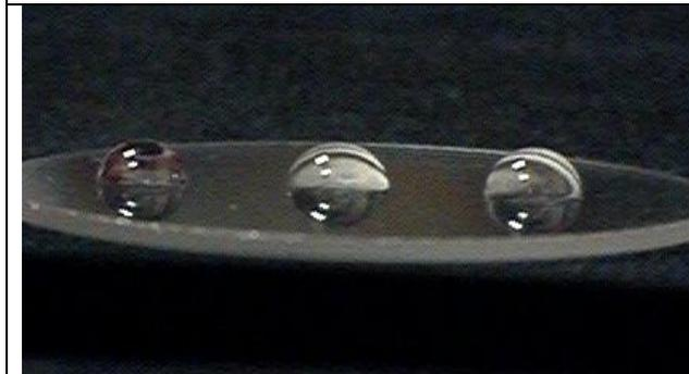
**Figure 7: Water droplets on an Al<sub>2</sub>O<sub>3</sub> coated window**
