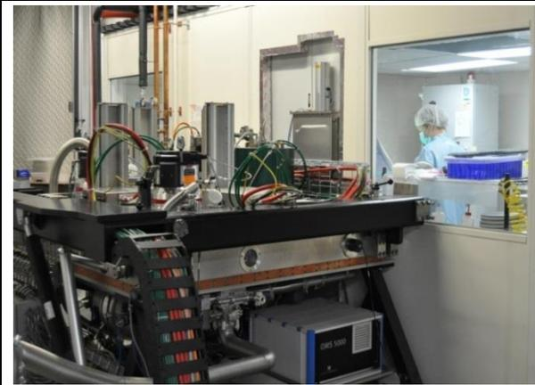
**Figure 11: The Helios multi-target high volume reactive sputtering coater provides high volume capability and reliable performance for the most challenging designs.**
