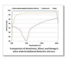
The Ultra-Wide series is Omega's most advanced and highest-performing broadband dielectric mirror, exhibiting uniformly high reflectivity from UV to NIR. Dielectric mirrors have many advantages over metallic coatings, including environmental stability, durability, and consistently higher reflectivity across a broader range of wavelengths.
