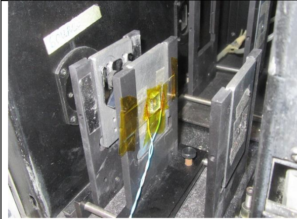
Figure 14: Filters were mounted on a glass strip coated with an ITO film. Voltage was applied across the strip.
