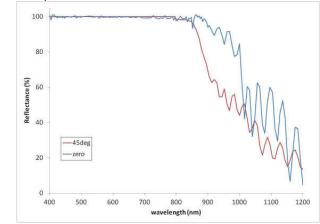
Broadband Sometimes an application requires high reflectivity over a wavelength range that spans several of those mentioned above. Such applications include hyperspectral imaging, astronomy and solar photothermal or photovoltaics. For the highest and flattest reflectivity response, dielectric mirrors can be designed (similar to our Ultra Broadband Dielectric Mirror)
