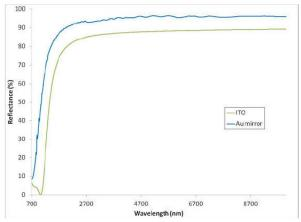
NIR – IR (700 nm- 10 micron) In the NIR and IR, gold mirrors are often used which absorb light in some visible wavelengths, but have high reflectance (>95% above 1500 nm). Another option is a transparent conductive oxide mirror (like ITO) which provides high reflectivity at longer wavelengths with transparency at shorter (visible) wavelengths.
