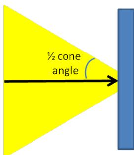
1/2 cone angle describes the beam convergence or divergence as it hits the filter.
