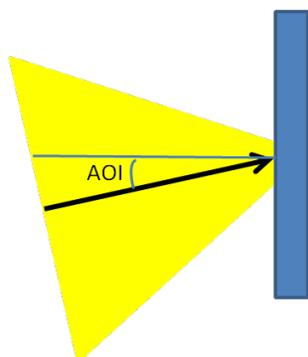
Angle of incidence (AOI) describes the angle of the primary beam and the normal to the surface of the filter.
