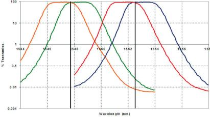
Transmission of 2 filters measured at 0° (Blue/Green) and 5° (Red/Orange) angle of incidence (AOI) using a scanning wavelength laser. The black lines locate the target C-band laser lines ITU 31 (1547.7 nm) and ITU 37 (1552.3nm). Top is linear scale to show the high transmission, Bottom is log scale to show blocking.
