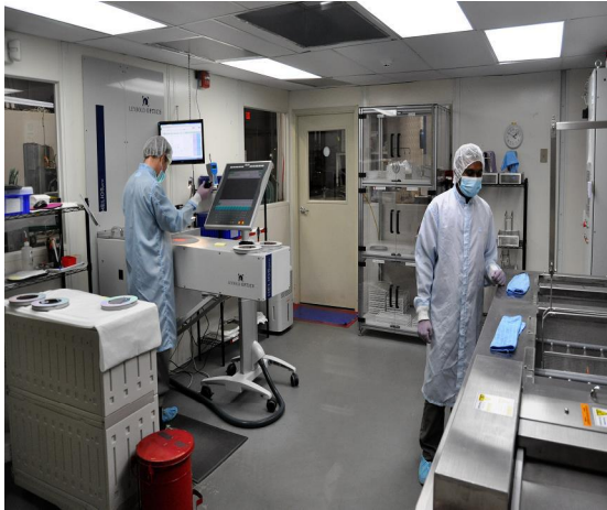
Figure 18: Parts and product are cleaned and handled in a clean room environment to ensure high yield and the most effective control of production cost.
