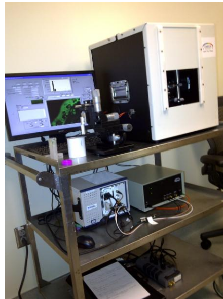
Figure 3. System photo: monitor, optical package, electronics box, quad core controller
