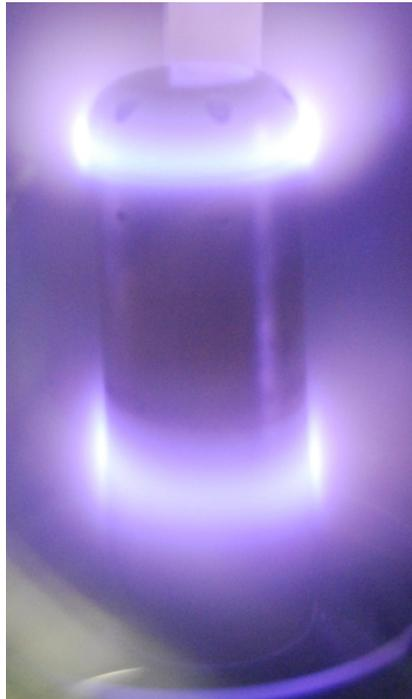
Figure 9: Separated unipolar magnet configuration (SMC)
