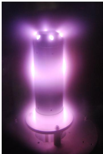
Figure 6: In the glow discharge region (poor vacuum) the electric field dominates.
