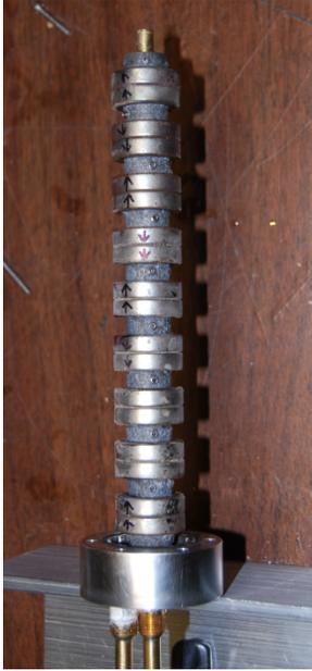
Figure 11: The configuration used for coating cylinders is shown. The polarity of each magnet set is flipped. A final magnet set is three magnets mounted in the nose piece.
