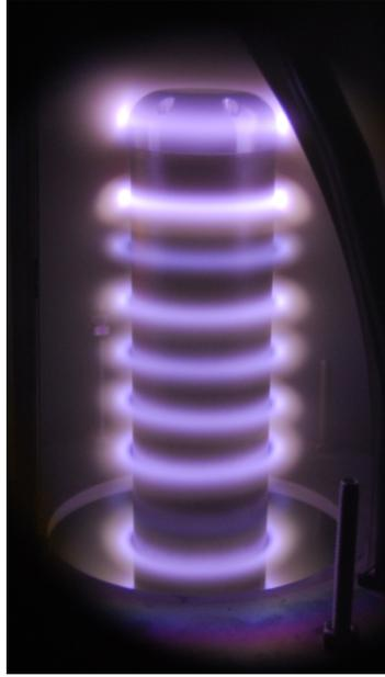
Figure 12: Each flipped pair creates a plasma ring. The bleed gases are argon and oxygen.
