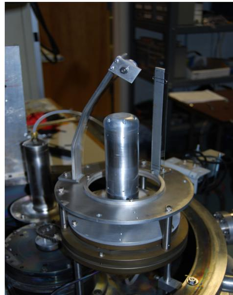
Figure 4: Aluminum cylindrical magnetron is shown in center of rotating tool, along with curved glass slide holder.
