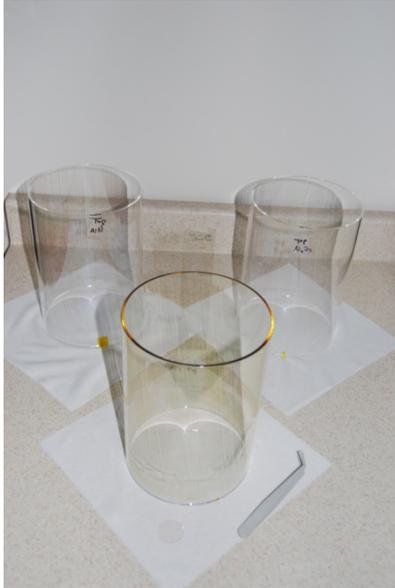
Figure 28: The back cylinders are coated with a single film of AlN (left) and Al<sub>2</sub>O<sub>3</sub> (right). The front cylinder is coated with the 6-layer AR design. It has a light yellow tint due to some absorption in the visible. The films exhibit good adhesion and film quality.
