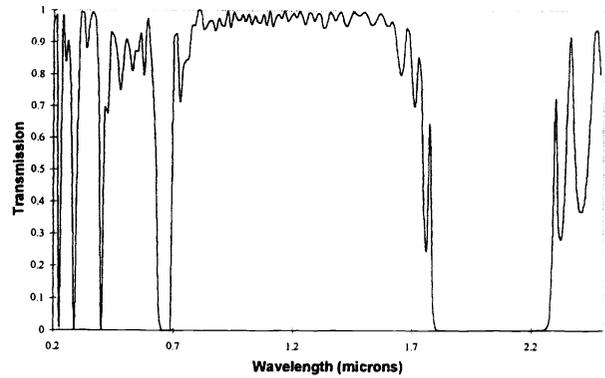
Figure 1b: Predicted performance for the discrete, quarter wave stack filter. The odd ordered harmonics at 0.66, 0.4, 0.28, and 0.22 microns are characteristic of discrete filters.
