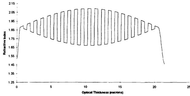
Figure 141a: Index profile for an amplitude modulated, apodized square wave filter. This design requires gradient index deposition.
