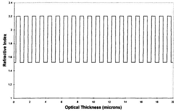
Figure 1a: Discrete index profile for a 2 micron quarter wave notch filter. The index contrast is what might be expected for a TiO<sub>2</sub>/SiO<sub>2</sub> film system.
