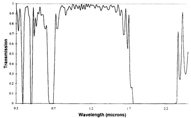
Figure 15b: Discrete, two material stack design. Materials and indices modeled are  $\text{TiO}_2$ : 2.3, and  $\text{SiO}_2$ : 1.46<sup>5</sup>.
