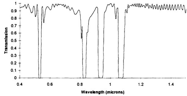
Figure 6b: Spectral performance for four notches produced in parallel at .532, .828, .935 and 1.064 microns.
