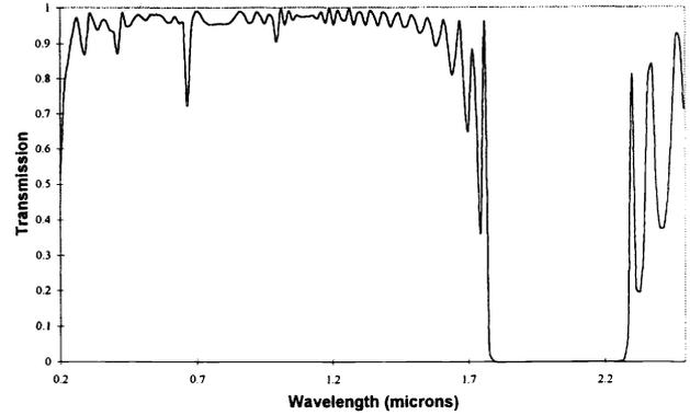
Figure 15c: Digitized five material stack design. Materials and indices modeled are  $\text{TiO}_2$ : 2.3,  $\text{Ta}_2\text{O}_5$ : 2.0,  $\text{Nb}_2\text{O}_5$ : 1.9,  $\text{Al}_2\text{O}_3$ : 1.67, and  $\text{SiO}_2$ : 1.46.
