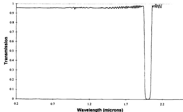
Figure 5b: Performance for sine and exponential sine wave Rugates for an index excursion of 0.1 are overlaid. The second harmonic is less noticeable at lower index excursions, and lower optical densities.
