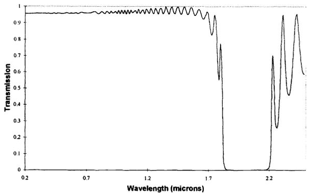
Figure 3b: Predicted performance for the Rugate, exponential sine gradient index filter. This waveform gives very good high order harmonic suppression.
