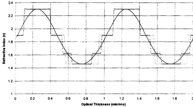
Figure 15a: A sine wave index profile can be initially designed, and digitized onto a discrete material matrix.
