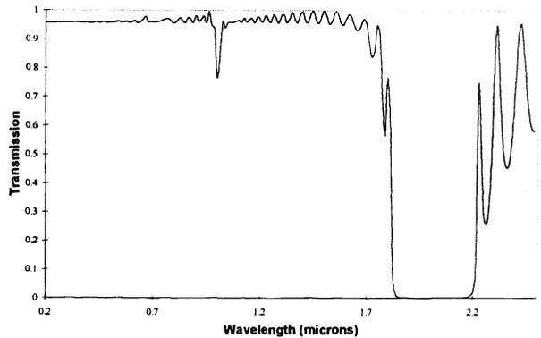
Figure 2b: Predicted performance for the Rugate, sine wave gradient index filter. The sine wave index profile exhibits good high order harmonic suppression, however, a weak, second order harmonic is present.
