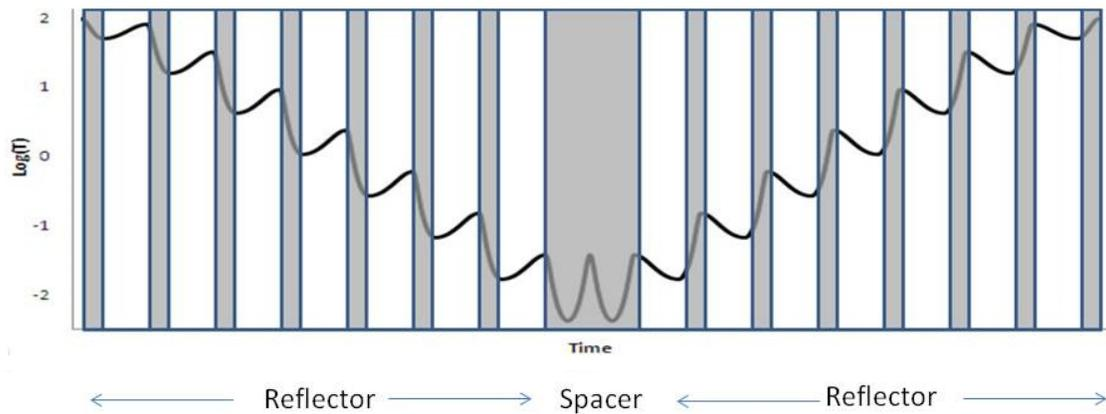
Figure 1. Stack Schematic and Theoretical Run Trace
