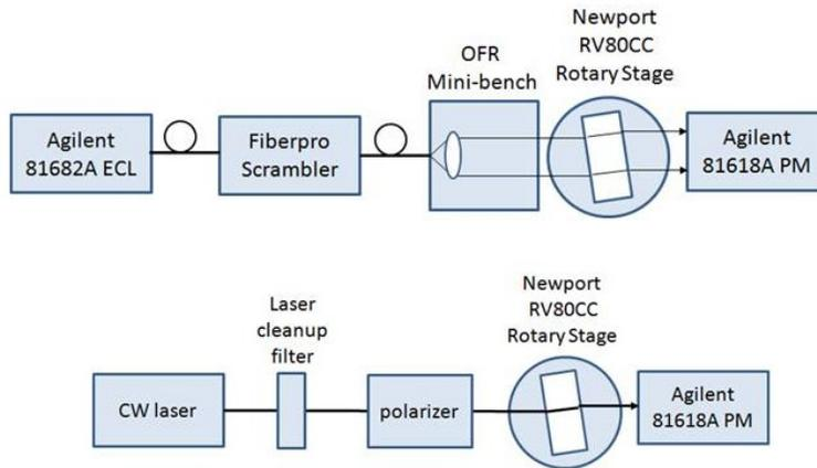
Figure 4. Laser Test Sets
