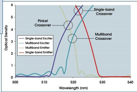
a 500-nm long-pass filter (the wavelength at 50 percent transmission) will achieve OD5 blocking (0.001 percent transmission) at 495 nm, or 500 nm minus 1 percent. Less demanding and less expensive designs have five-decade slope factors of 3 to 5 percent. Designs and manufacturing technologies produce filters of radically different band shape and throughput, allowing application-specific properties.
