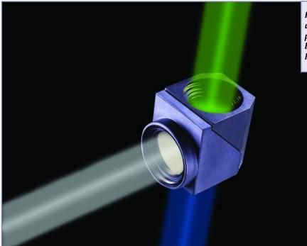
for conventional fluorophores such as DAPI (blue), fluorescein (green) and rhodamine/Texas red (orange/red). Two- and three-color sets are most common, while the fourth "color" in a four-color set includes a fluorophore in the 650- to 800nm range. Multiple passbands limit the deep blocking achieved in single-band filter sets, resulting in a lower signal-tonoise ratio from multiband sets.
