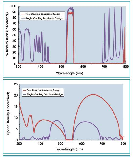
Figure 3. In the theoretical transmission of two bandpass designs (top), the differences in passband transmission are moderate, but the out-of-band transmission is more attenuated using the two-coating design. The corresponding theoretical blocking curves (bottom) show that the single-coating design has moderate near-band blocking, while the short-pass/long-pass design has deeper and more extensive blocking.
