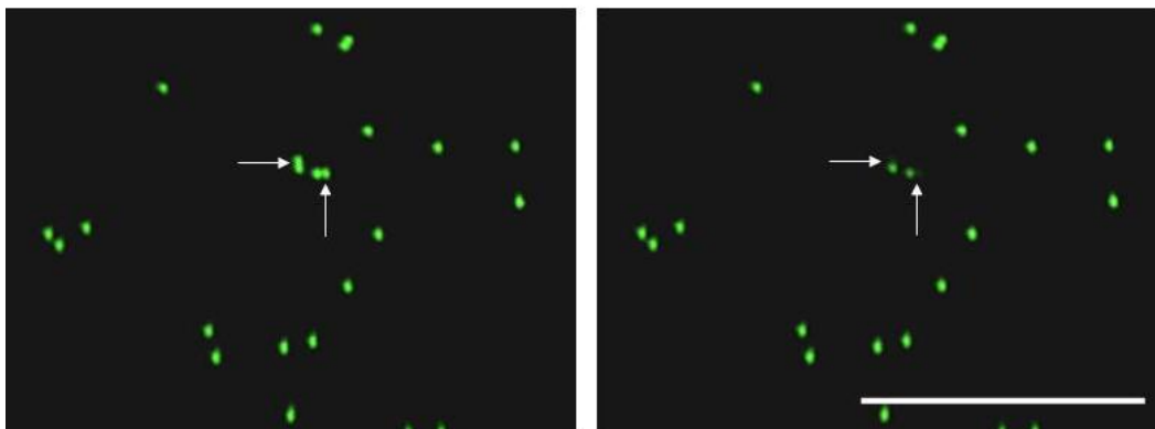
Figure 3. Microscopy of fluorescent beads before (left) and after (right) selective laser ablation of two beads marked with arrows (scale bar is 100 \mu\text{m} )
