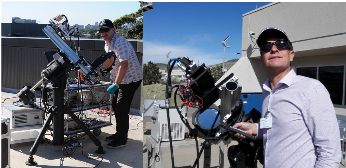
Figure 6. Mark Keevers and the spectrum-splitting CPV prototype during outdoor testing at UNSW (left) and NREL (right).
